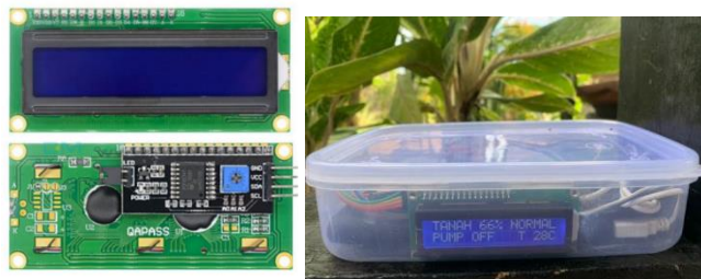
Gambar 10. LCD 16x2 I2C
